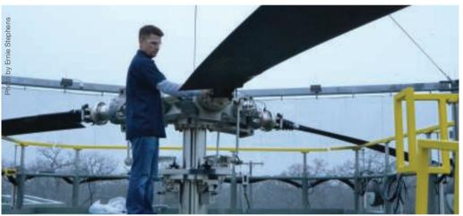
A technician inspects a blade mounted on CTI's new whirl tower. The system uses computers and lasers to compare test blades to a perfect "master" at operational rotation speeds.
