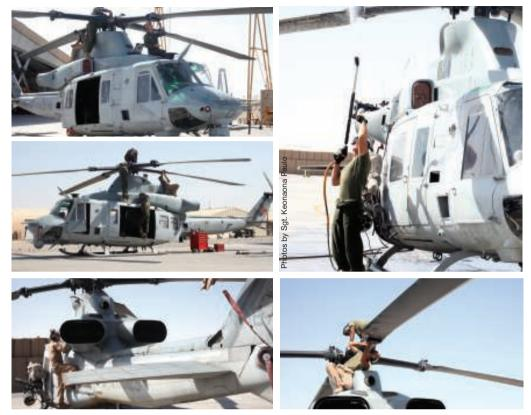
U.S. Marines with the Marine Light Helicopter Squadron (HMLA) 469, Marine Aircraft Group 39, 3D Marine Aircraft Wing (Forward) stationed at Camp Bastion, Helmand province, Afghanistan perform routine maintenance on a Bell UH-1Y Venom. Mechanics repaired the rotor and washed the helicopter as part of aviation readiness for the 469.
