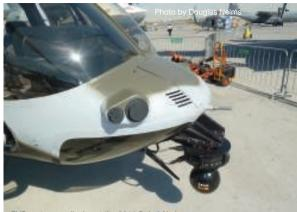
FLIR system on display at the 2011 Dubai Airshow.
