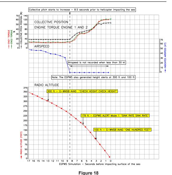
EGPWS Simulation with Mode 1 alert triggered at 179 ft
