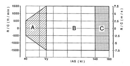
Figure 5 (A + B + C) = Complete IFR flight envelope
